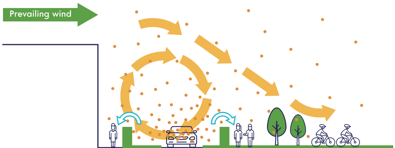
Figure 4. Protecting people with hedges at the side of an open road Source: Greater London Authority, 2019
